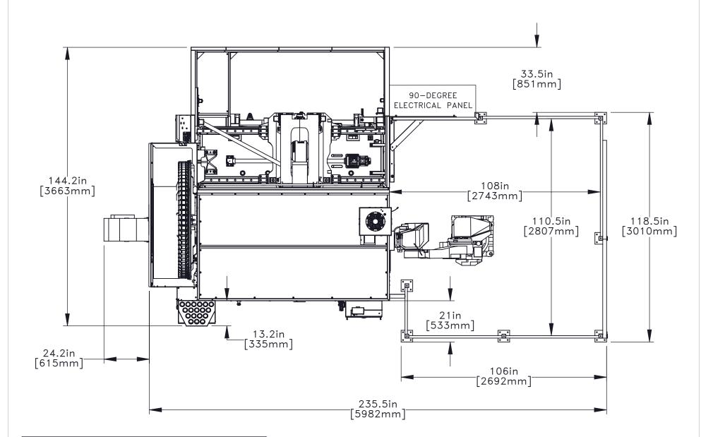
CONVEYOR DISTANCE SHOWN WITH BELT-TYPE CHIP CONVEYOR. OTHER CONVEYOR TYPES ADD MORE LENGTH
